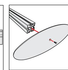
**Base Plate & Extrusion Connection**
